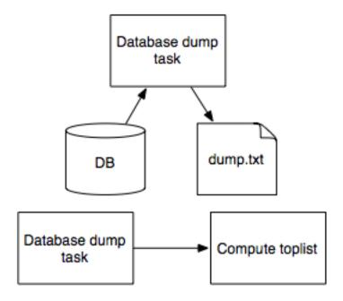
Each task defines its outputs using the output() method. Additionally, there is a helper method input() that returns the corresponding Target classes for each Task dependency.
